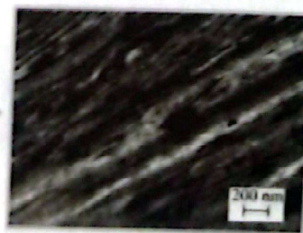
Intermediate structure: fine lamellae of Fe and Pt with A1 FePt at their interfaces
