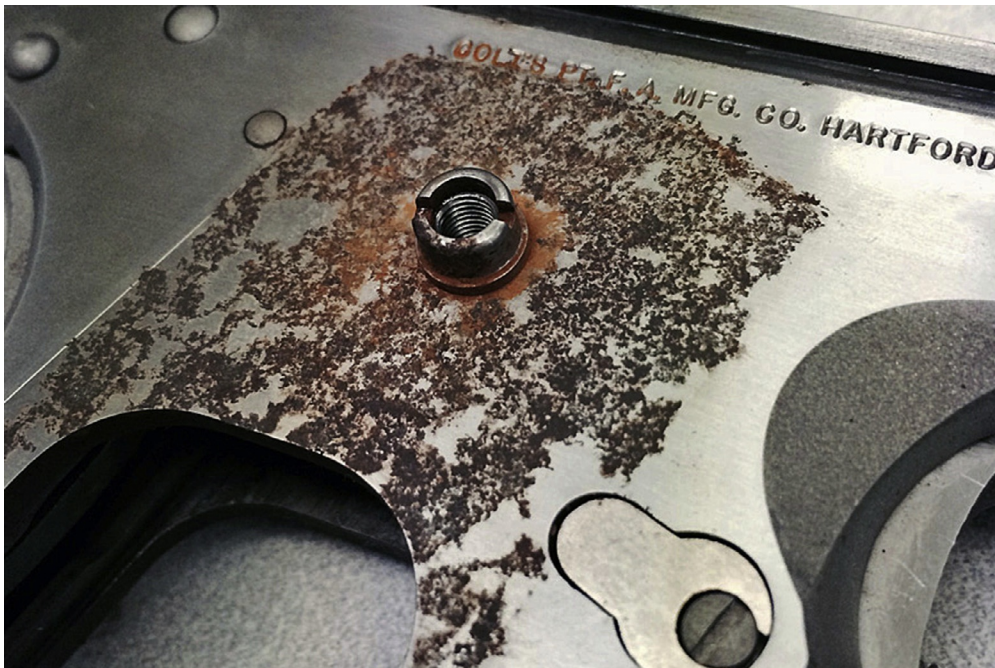
Fig. 1.8 Galvanic corrosion of stainless steel under grip panel area in Series 80 Colt Gold Cup 1911 pistol [22]. http://ravelingroup.com/wordpress1/tag/colt-gold-cup/ .
