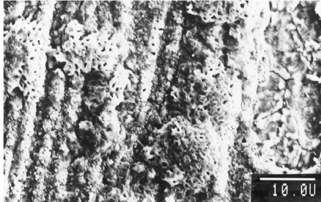
Fig. 11.25 Oxide surface with Mo-implantation after 48 h of exposure to air at atmospheric pressure and 1173 K [64].
