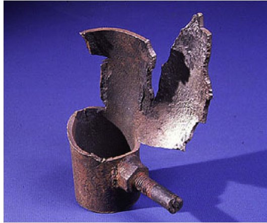
Fig. 1.18 Rupture caused by hydrogen embrittlement [51]. http://www.gewater.com/handbook/boiler_water_systems/fig14-10.jsp0 .
