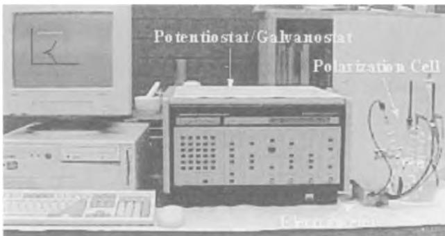
**Figure 6.3 Modern electrochemical instrumentation.**
