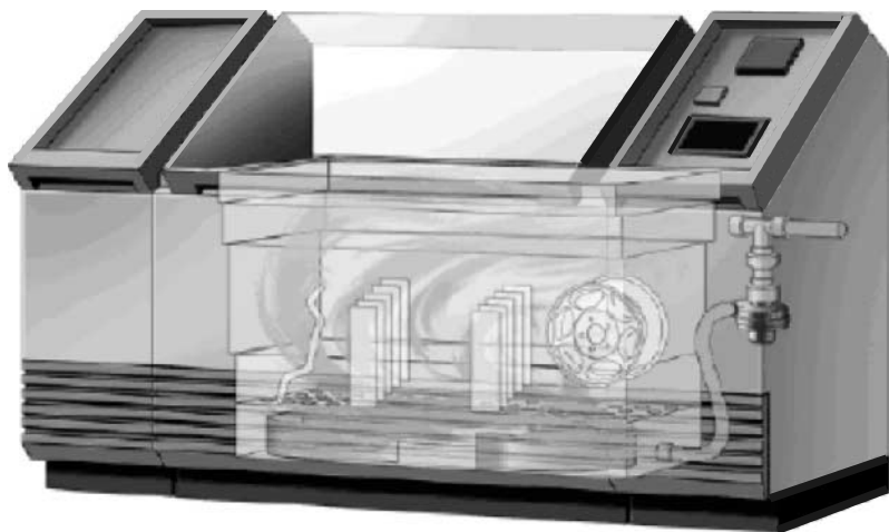
Figure 7.14 Controlled salt fog test chamber during a dry cycle.
