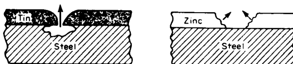
Figure 3-6 Galvanic corrosion at perforation in tin- and zinc-coated steel. Arrows indicate corrosive attack.
