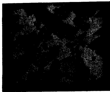
Figure 3-26 Electron photomicrograph of carbides isolated from sensitized type 304 stainless steel (13,000 \times ).
